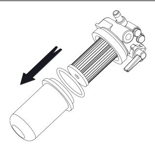
Slide down the casing bowl (4) to expose the filter element (2). Ensure that the O-ring seal (5) is also removed from the assembly.
