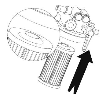
Insert a new filter element (2) up into the base (1). Ensure the central opening of the filter is firmly pressed against the base. When installed correctly filter should hang from the base on its own.
