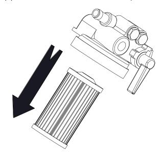
Remove the filter element (2) from the assembly by pulling it downwards. In the event that metal flanges separate from the filter element, ensure they are removed as well.
