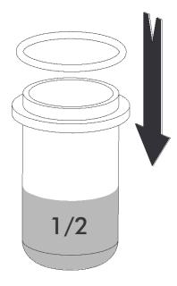
Install the O-ring seal (5) over the casing bowl (4). Seal should have a tight fit, if loose replace the O-ring seal. Fill the casing bowl (4) with clean diesel fuel no more than half way.
