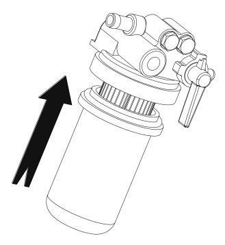
Install the casing bowl (1) fitted with an Oring seal (5) over the filter. Seal should be seated against the base (1).
