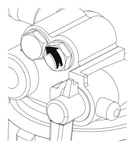
Loosen the vent screw (7) by  $\frac{1}{2}$  turn in the indicated direction. Vent screw should not be completely removed.
