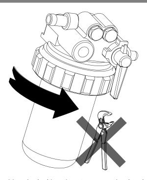
Position the locking ring (3) over casing bowl (4). Take special care in aligning threads and screw on the locking ring finger tight. Ring should turn freely when threads are properly engaged. Tighten the locking ring (4) hand tight. DO NOT USE PLIERS OR ANY OTHER TOOL TO TIGHTEN THE RING.
